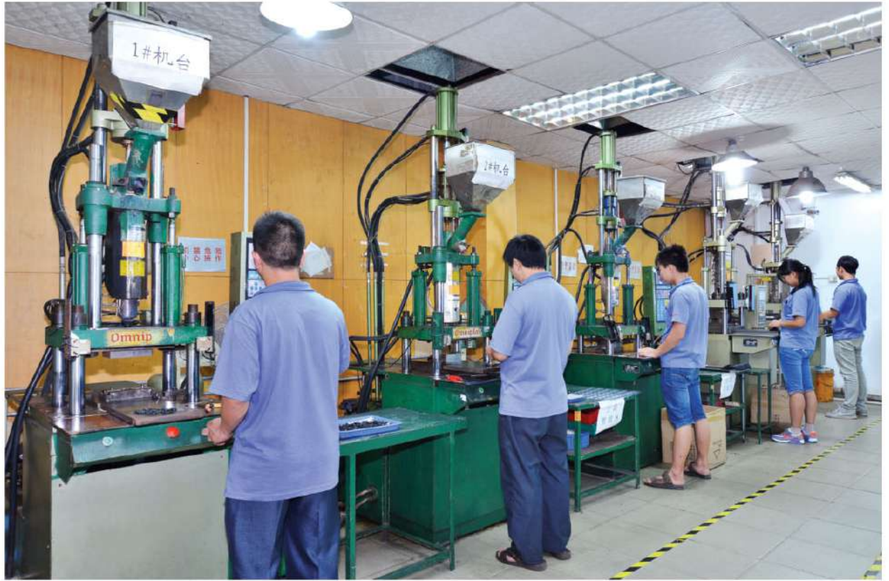
注塑車間 Plastic injection workshop
